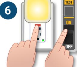
Press the **RESET** button or switch the breaker to the **on position** – the device should **turn back on**
