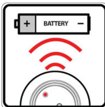
Smoke alarm batteries should be replaced at least once a year. If an alarm "chirps" or beeps to indicate low batteries, they should be replaced immediately.
